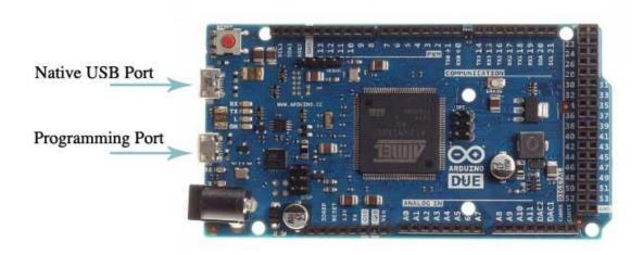
Either of the USB ports can be used for programming the board, though it is recommended to use the Programming port due to the way the erasing of the chip is handled:
