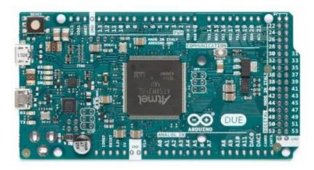
The Arduino Due is a microcontroller board based on the Atmel SAM3X8E ARM
