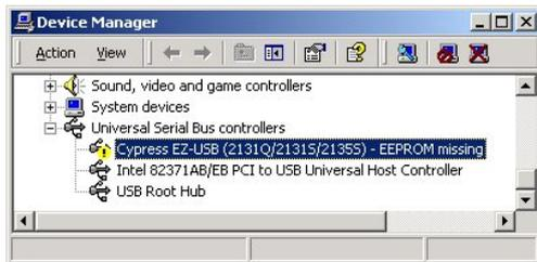
Figure 18 USB Driver was not installed correctly.
