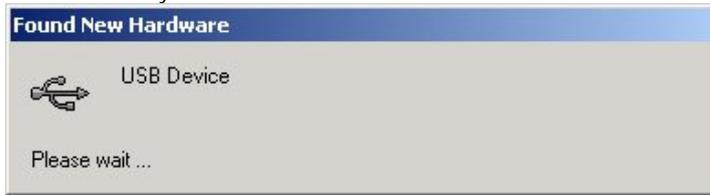
When prompted for an installation file, refer to the file "ezusbw2k.inf" that was extracted during the demoboard software installation (step 1) in the directory of your choice (default C:\program files\austramicrosystems AG\AS5046\_DemoBoardSW\_x.x).
