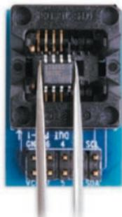
Align PIN 0 of the SOIC package towards the header-pins side of the adaptor board.
