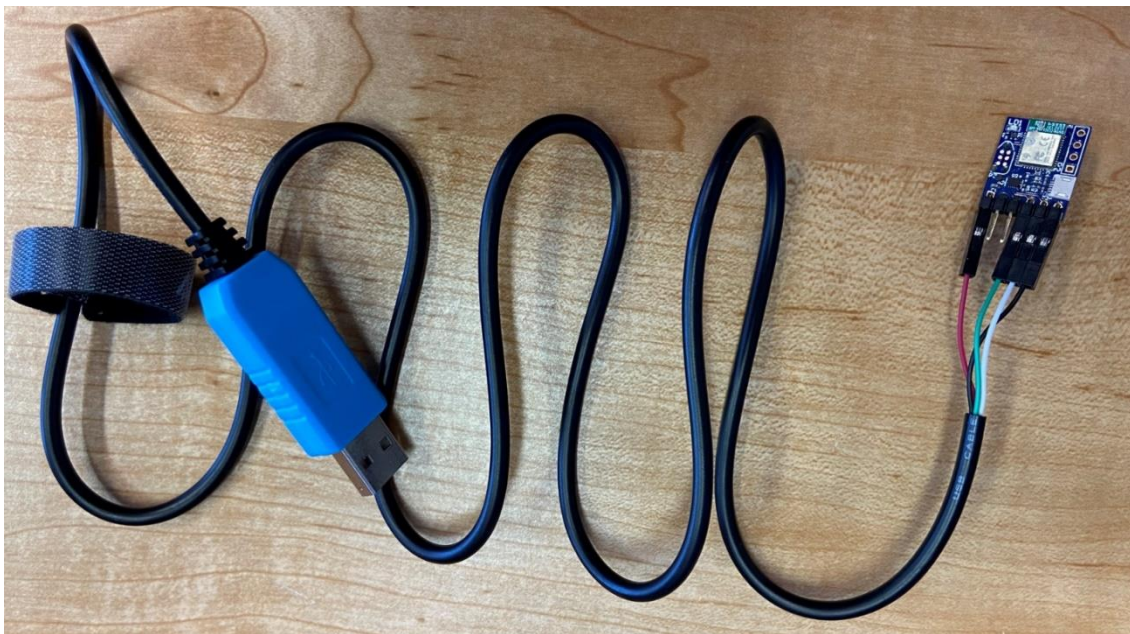
Fig. 7. Connect BlueIO832Mini with a USB-UART adapter. The 5V and GND wires can be used for powering BlueIO832Mini thanks to its internal level shifter.
