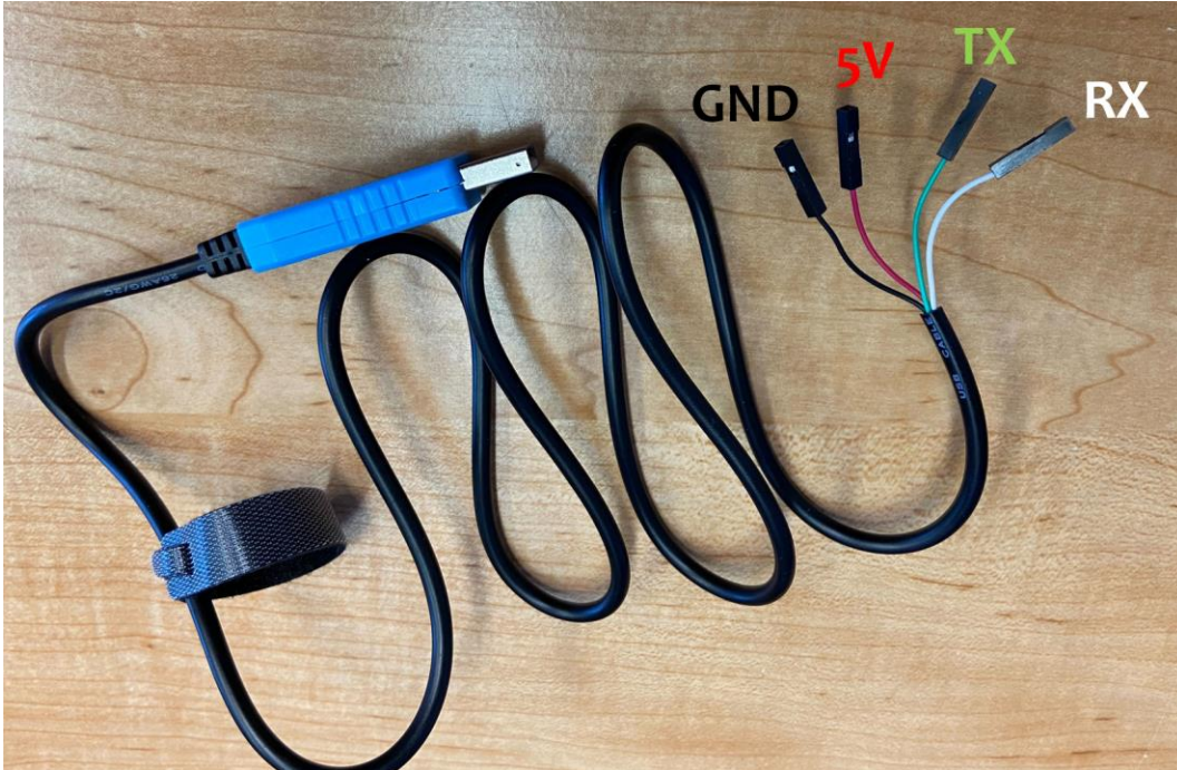
Fig. 5. UART's pins on USB-UART adapter. UART-TX (Green), UART-RX (White), 5V power supply (Red), and Ground (Black)
