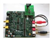
Connect an audio source (CD-player, MP3-player or similar) to the line-in input of the AudioEB with CC85xxEM or CC85xx-CC2590 with the "MASTER" label plugged in.
