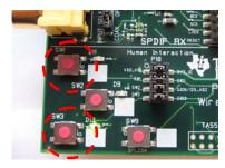
The output volume can be adjusted on the Slave by pressing SW 1 to increase the volume and SW3 to decrease the volume.
