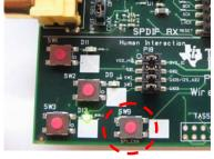
When powered for the first time, LED D9 will blink to indicate that the devices are not connected
