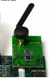
Connect the CC85xxEM or the CC85xx-CC2590EM marked MASTER (label attached on the backside of the board). These boards are pre-programmed with master firmware. Attach the antenna to the SMA connector.
