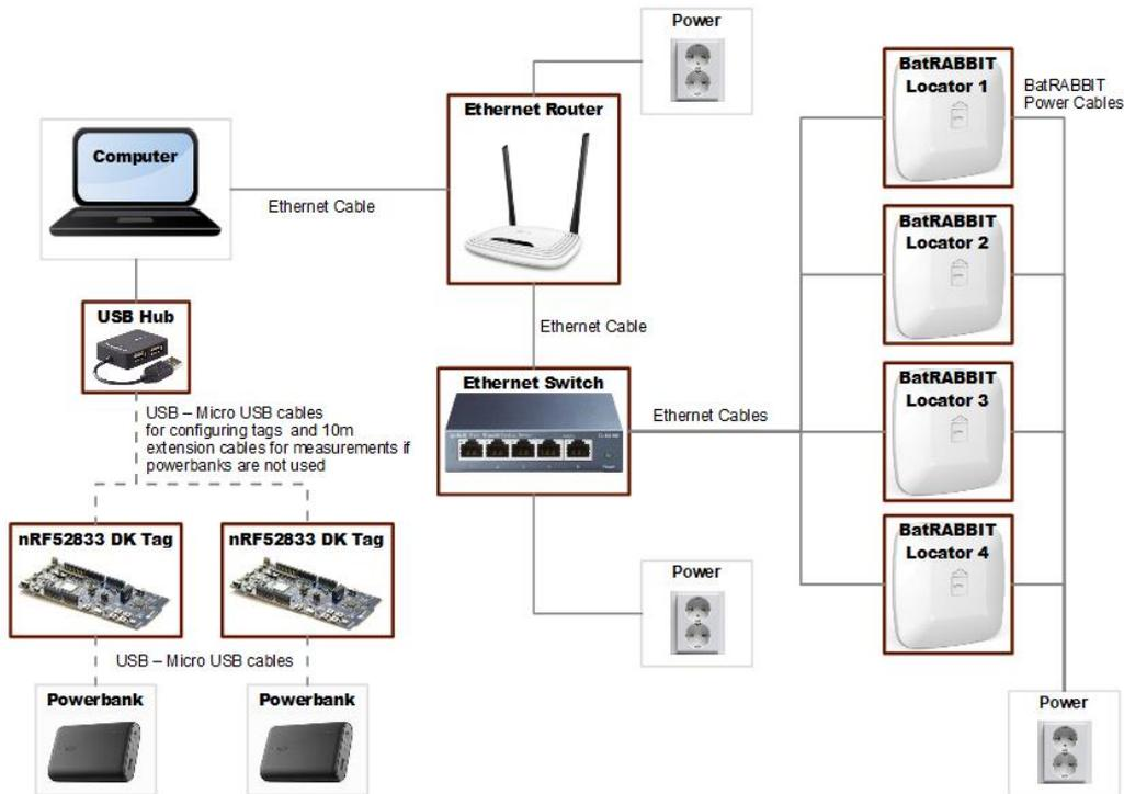
Gen2 locators can be installed e.g. on ceiling (mounting on floor, wall, 45 degrees from floor and 45 degrees from ceiling are also supported) of a room and connected via Ethernet to Windows 10 PC running proprietary CoreHW AoA Demo software. PC Demo software can be used to demonstrate AoA Tag position estimation based on Angle-of-Arrival data.
