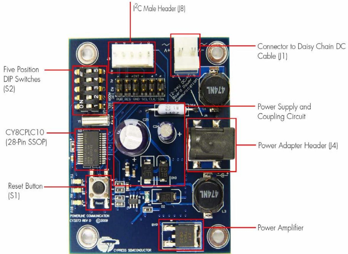
The communication signal flow on this LV board is:
