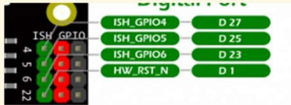
For example: GPIO Pin 4 on board >> ISH\_GPIO4 >> D 27, so the pin number in the code should be 27.
