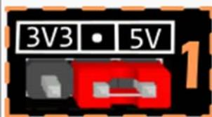
Jumper cap for switching voltage
