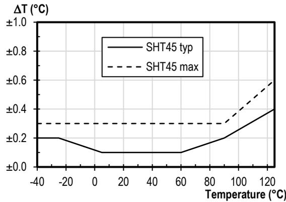
**Figure 10:** SHT45 typical and maximal temperature accuracy.
