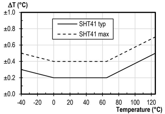
**Figure 9:** SHT41 typical and maximal temperature accuracy.
