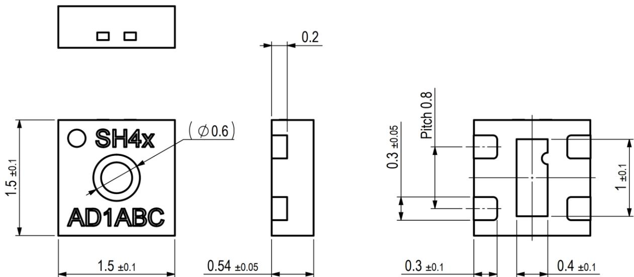
**Figure 12** Dimensional drawing of SHT4x including package tolerances (units mm).
