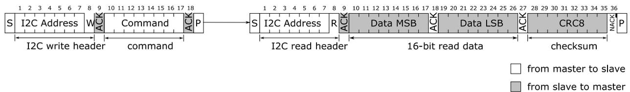
**Figure 11:** I2C transfer types: First a write header is sent to the I2C slave, followed by a command, for example “measure RH&T with highest precision”. After the measurement is finished the read request directed to this I2C slave will be acknowledged and transmission of data will be started by the slave.
