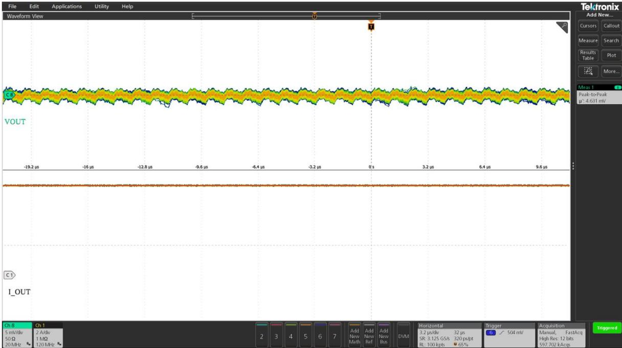
Figure 14  $V_o$  ripple at 12A (Ch1: $I_o$ , Ch8:  $V_{OUT}$ ), peak-peak  $V_o$  ripple = 4.6mV
