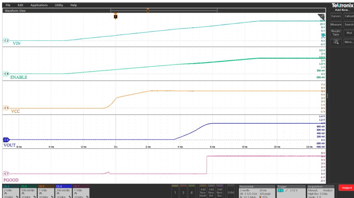
**Figure 9 Startup with 12A load (Ch2:PV<sub>IN</sub>, Ch5:V<sub>CC</sub>, Ch6: V<sub>OUT</sub>, Ch7: PGood, Ch8: Enable)**
