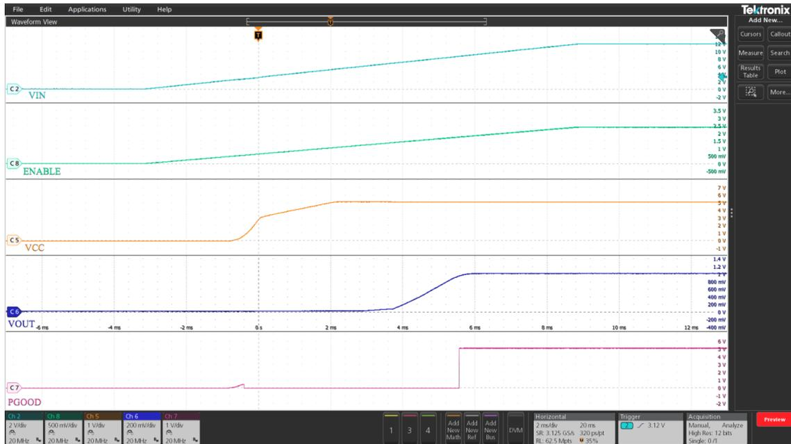
**Figure 8 Startup with no load (Ch2:PV<sub>IN</sub>, Ch5:V<sub>CC</sub>, Ch6: V<sub>OUT</sub>, Ch7: PGood, Ch8: Enable)**
