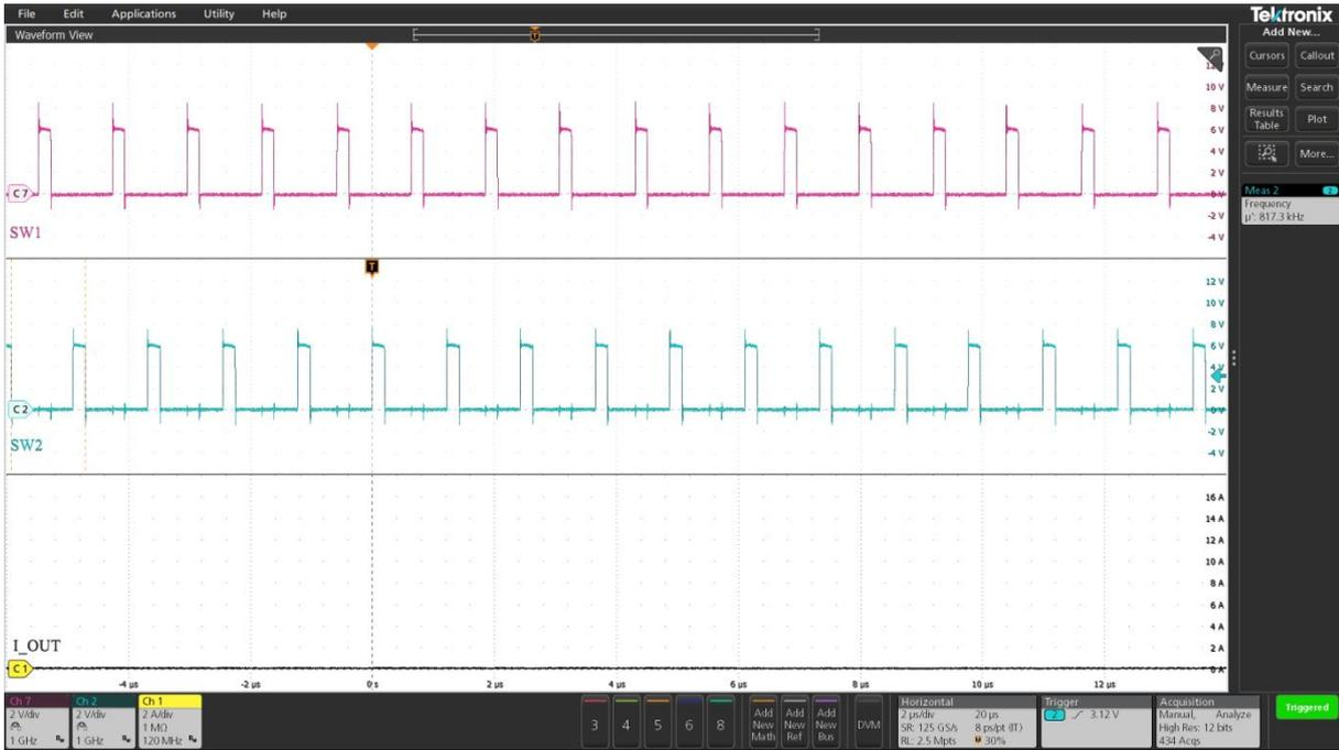
**Figure 12** Switch node waveforms at no load
