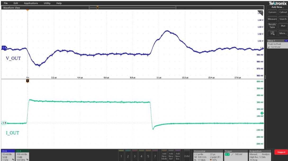
Figure 15 Transient response 0A to 6A (Ch6:  $V_{OUT}$ , Ch8: $I_o$ ), peak-peak deviation = 53mV, load slew rate = 40A/ $\mu$ s
