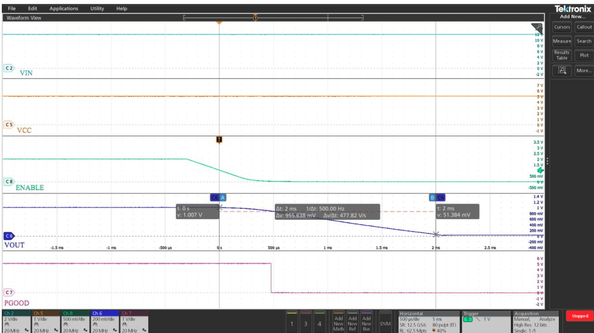
**Figure 11 Soft turn off at no load (Ch2:PV<sub>IN</sub>, Ch5:V<sub>CC</sub>, Ch6: V<sub>OUT</sub>, Ch7: PGood, Ch8: Enable)**
