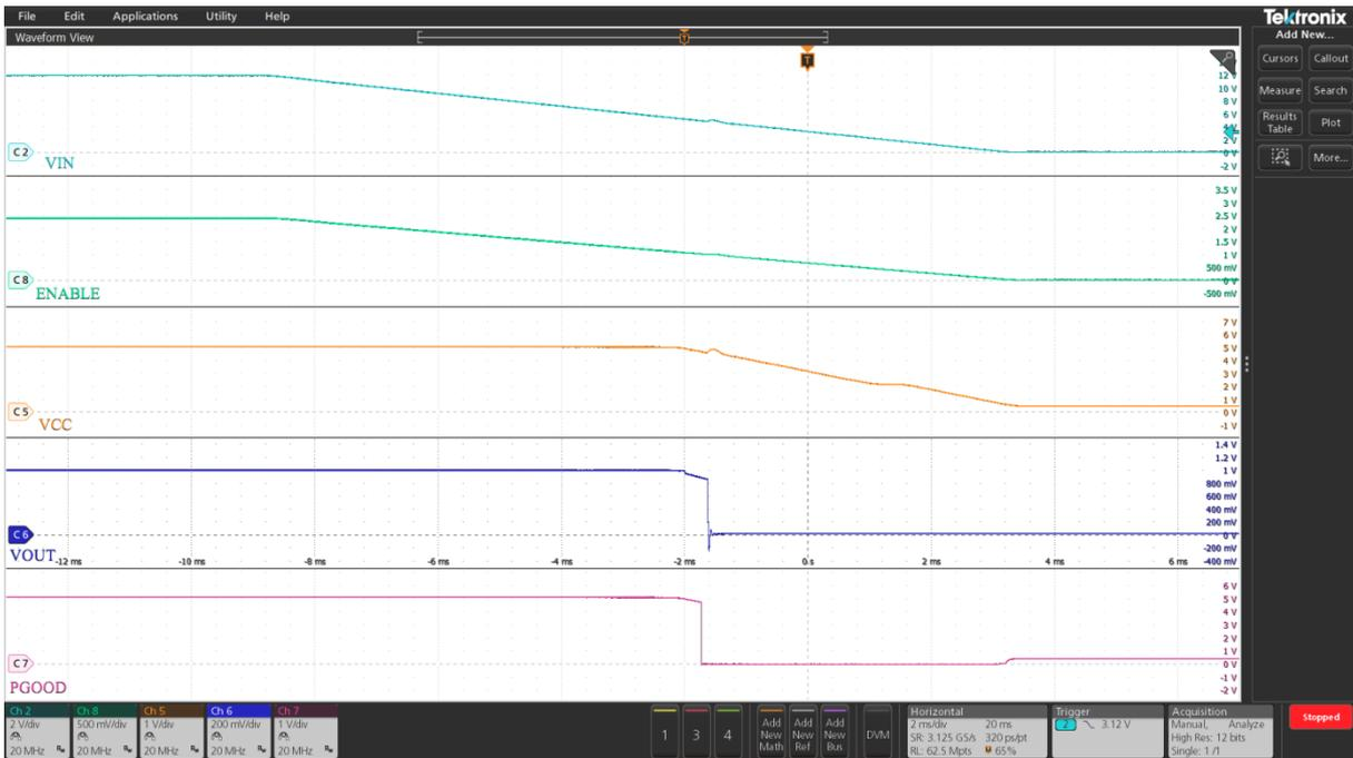
**Figure 10 Shutdown with Enable de-assertion at 12A load (Ch2:PV<sub>IN</sub>, Ch5:V<sub>CC</sub>, Ch6: V<sub>OUT</sub>, Ch7: PGood, Ch8: Enable)**
