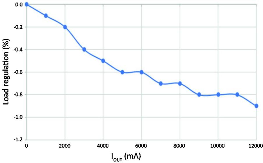
Figure 18 Load regulation ( $I_o = 0-12A$ )
