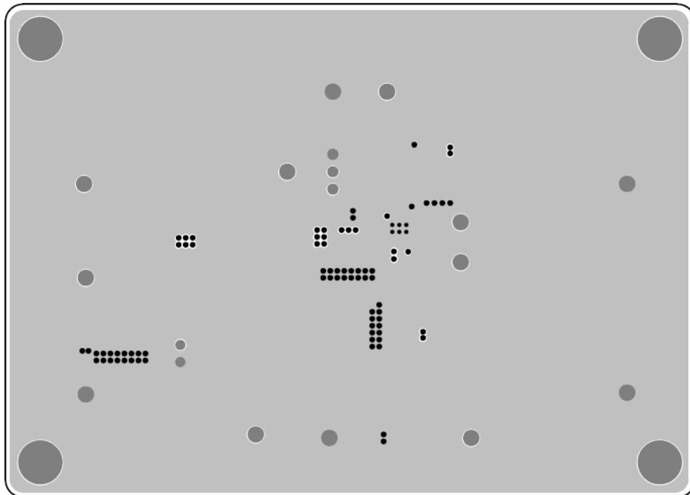
Figure 3. PCB Layout—Inner Side (3<sup>rd</sup> Layer)
