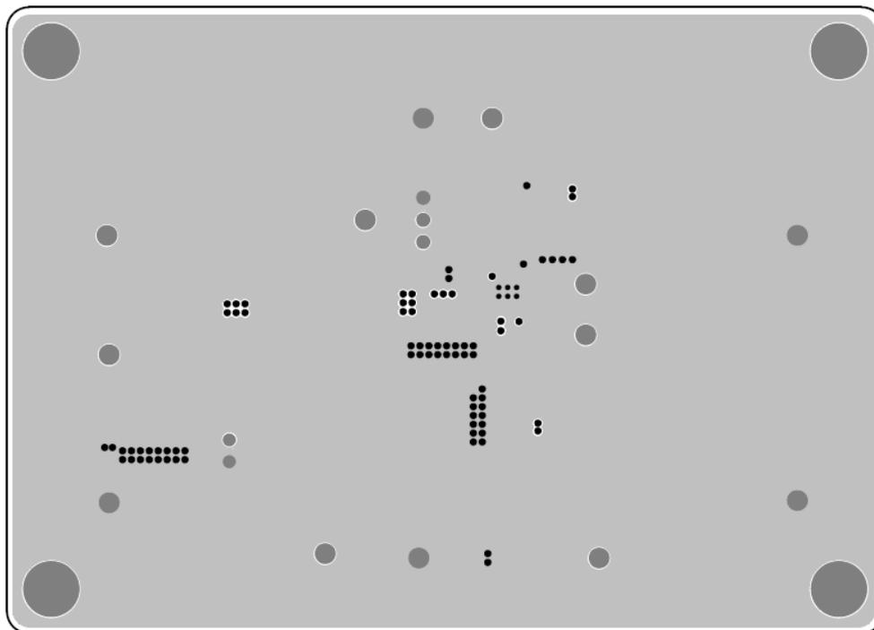
Figure 2. PCB Layout—Inner Side (2<sup>nd</sup> Layer)
