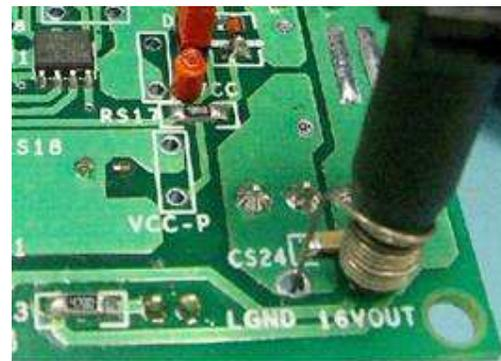
**Fig. 4D Recommended probing of Vout's Ripple & Noise voltage.**
