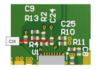
SS time is set at default of 1 msec. Adding a small MLCC capacitor between REF and RTN can extend the soft start time.
