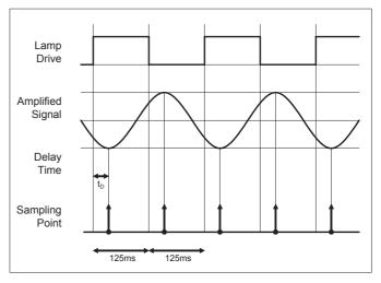
On some sensors where there is a difference in output level between the active and reference channels there will be a difference in delay time for each channel. In this situation the delay time should be set to the average value. The following section explains how to set the ADC measurement delay time and other sensor specific parameters.
