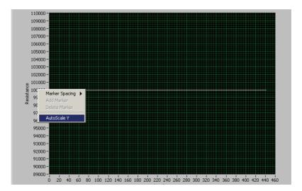
This stops the axis from automatically expanding.
