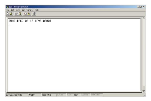
Note that if the Evaluation Kit is already set in 'Measurement Mode' then a data packet will be displayed once per second. A full list of HyperTerminal commands can be found in Section 16.
