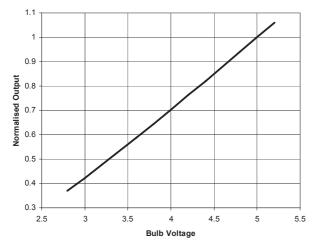
Pyro Output Voltage vs. Lamp Supply (IR12GJ Active Channel, Normalised at 5.0 V)
