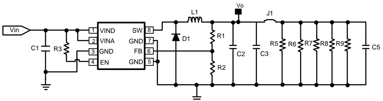
Figure 1. LM2832Y 8-Pin MSOP-PowerPAD Demo Board Schematic
