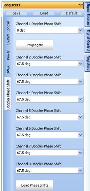
Use the pull down menus to select phase rotation angles for each channel individually or click on the “Propagate” button to duplicate the angle for all channels. Click on the “Load Phase Shifts” button.
