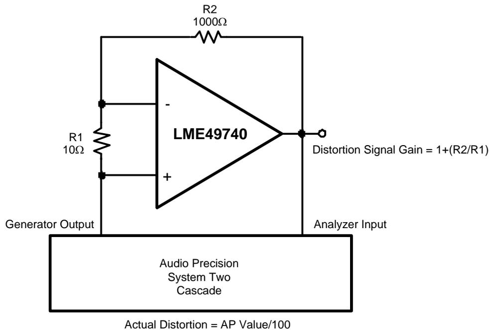
**Figure 23. THD+N and IMD Distortion Test Circuit**
