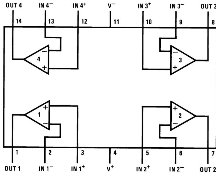
**Figure 2. 14-Lead SOIC (D Package)
