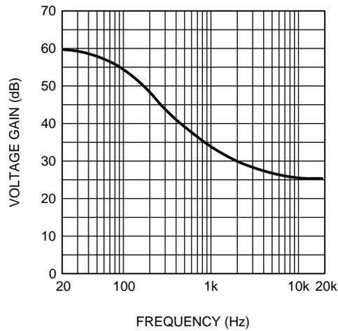
Figure 28. NAB Preamp Voltage Gain vs Frequency
