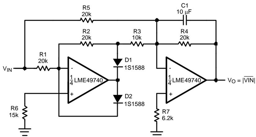
Figure 35. AC/DC Converter
