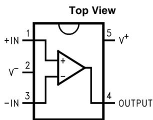
Figure 59. 5-Pin SC70-5/SOT-23-5 Package
