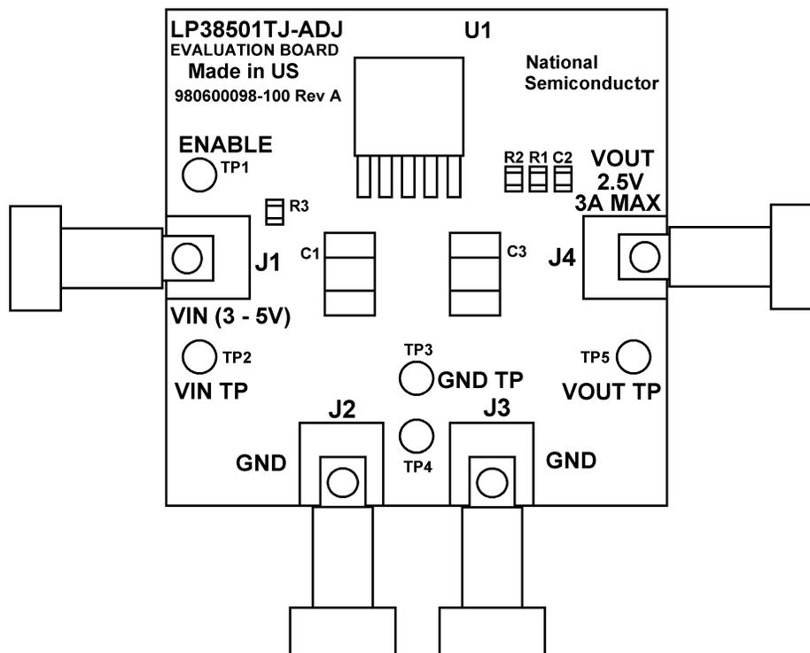
Figure 2. Top View of the PCB Assembly
