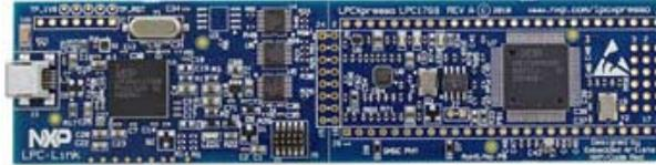
The LPC1768 LPCXpresso board with NXP's ARM Cortex-M3 microcontroller has been designed to make it as easy as possible to get started with Cortex-M3. The LPCXpresso comprises a target board combined with a JTAG debugger. A free Eclipse-based IDE from Code Red is also included.
