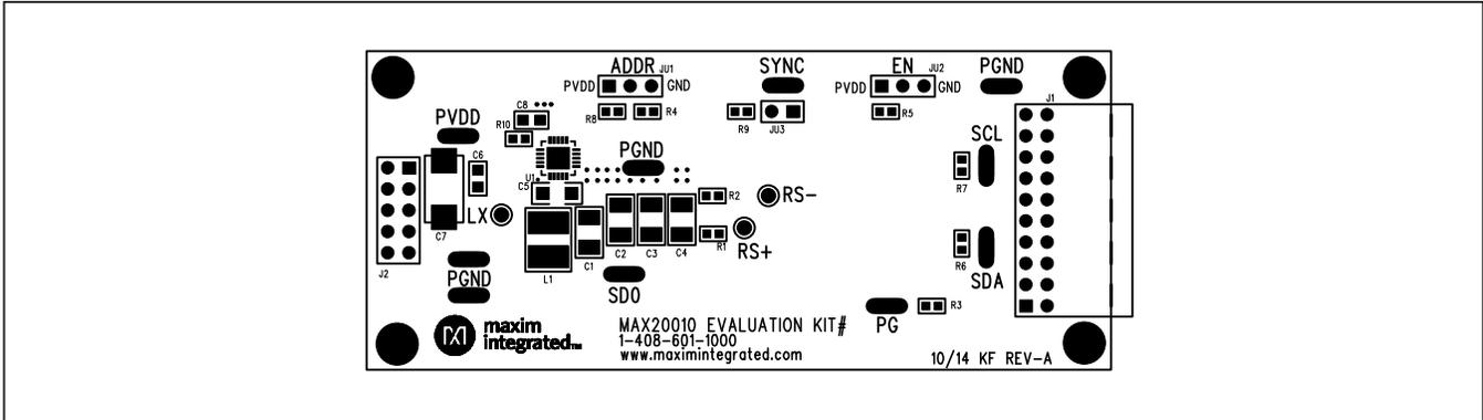
Figure 2. MAX20010 EV Kit Component Placement Guide—Component Side
