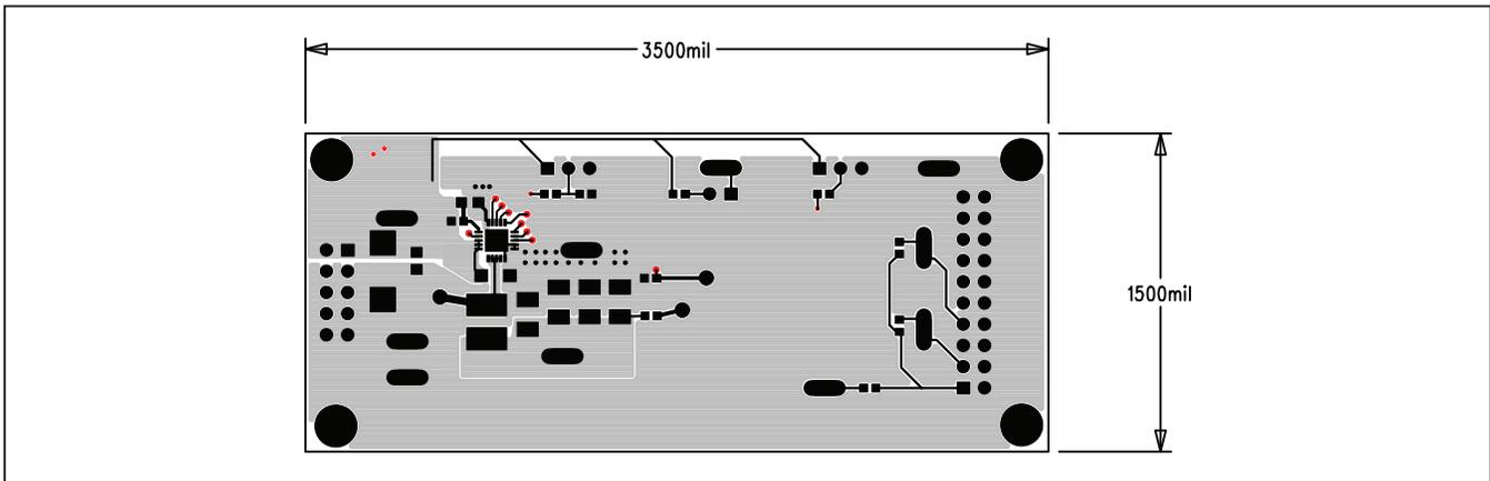
Figure 3. MAX20010 EV Kit PCB Layout—Component Side
