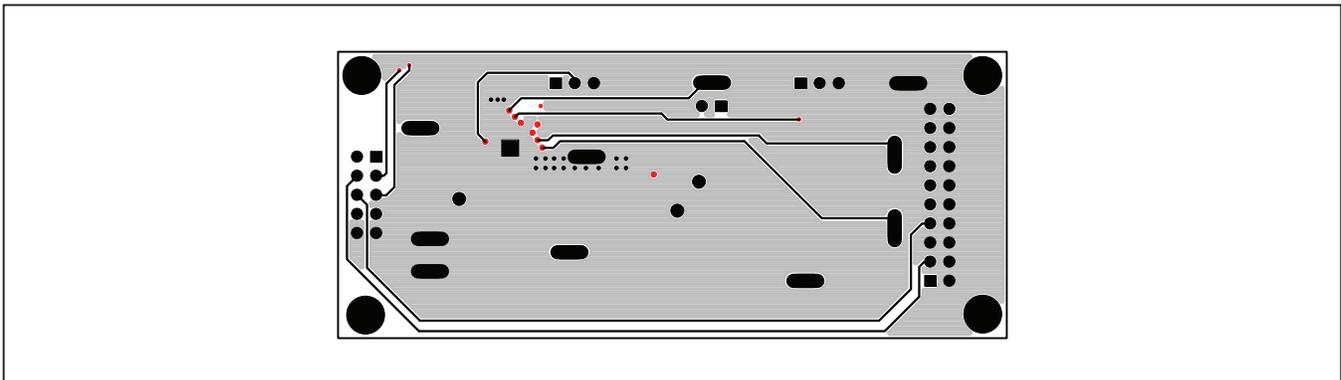
Figure 4. MAX20010 EV Kit PCB Layout—Layer 2
