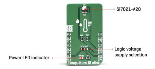
Each sensor contains the factory calibration data in the internal non-volatile memory, so there is no need for additional calibration steps. The datasheet of the Si7021-A20 offers conversion formulas, which should be used to convert the readings from the sensor to physical values, expressed in %RH and °C.
