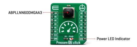
The sensor itself is based on a piezoresistive silicon membrane sensitive to pressure, which is backed up by an ASIC. The ASIC applies temperature compensation and calibration to the signal. The ratiometric voltage at the output pin is updated once per one ms (1kHz), allowing it to be used either by the A/D converter of the host MCU or directly within the control feedback loop, ensuring the least possible latency.
