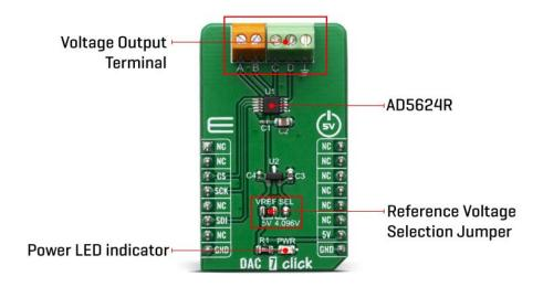
The DAC 7 click has a high precision voltage reference included onboard. For that purpose we have used 4.096V precision voltage reference MCP1541 from Microchip. This little SOT23 device is stable with capacitive loads. It has regulations for both sink and source and is very accurate. This gives DAC 7 click good flexibility for use in various applications.
