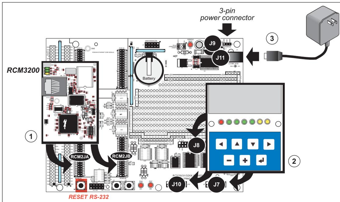
**Figure 2. Install the Modules on the Prototyping Board**
