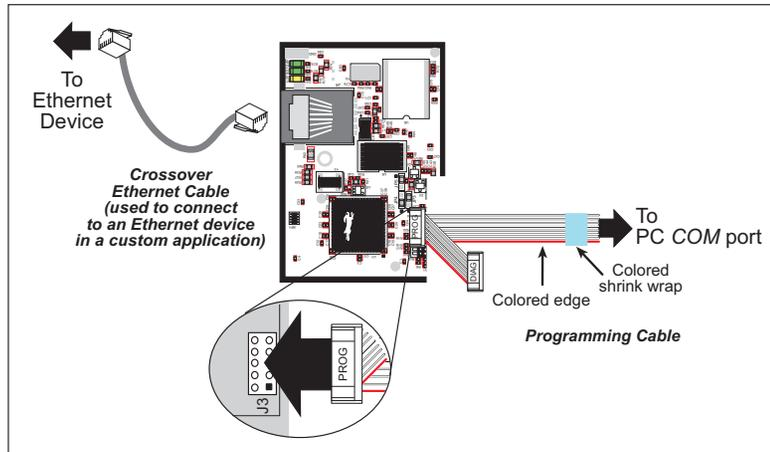
Figure 3. Connect Programming and Ethernet Cables to PC
