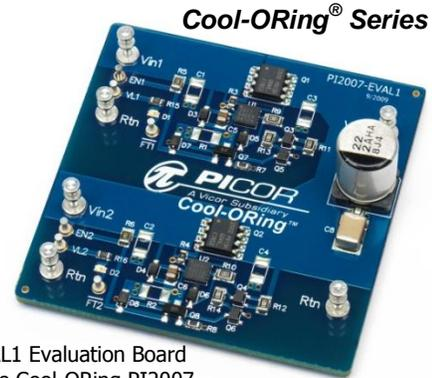
PI2007-EVAL1 Evaluation Board featuring the Cool-ORing PI2007 Active ORing controller.
