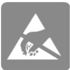
Proper ESD handling procedures must be followed throughout the mounting, handling and operation of any devices and equipment that incorporate the module to avoid ESD damages.
