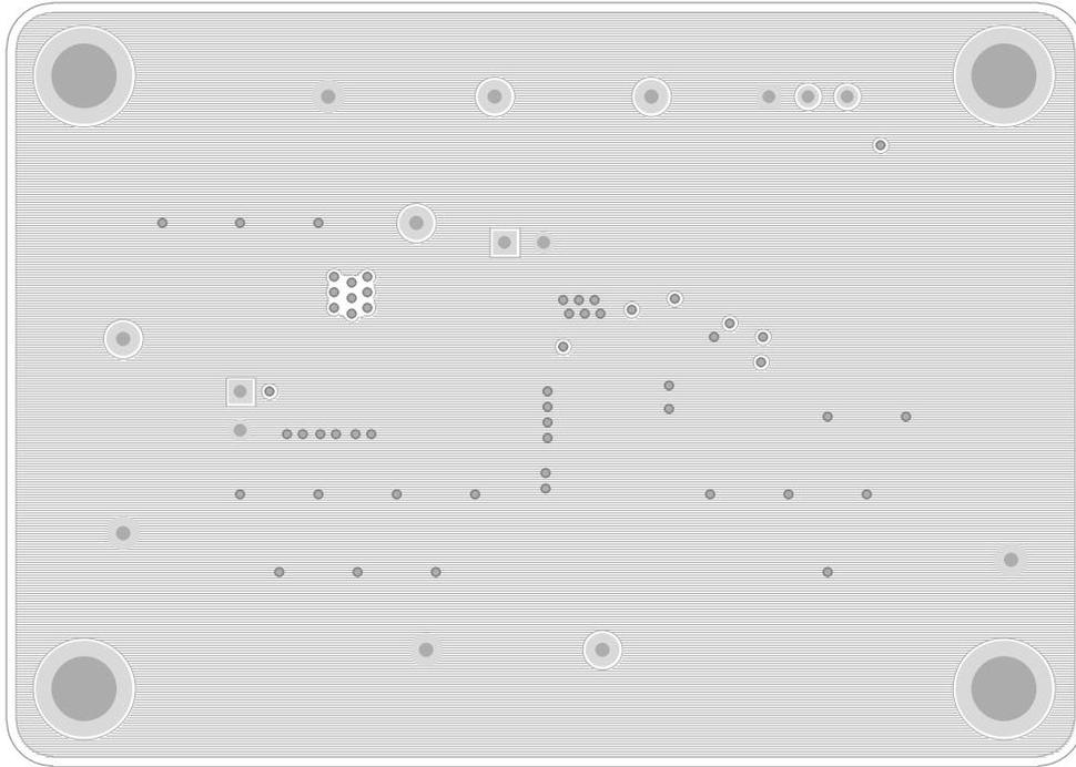
Figure 3. PCB Layout—Inner Side (3<sup>rd</sup> Layer)
