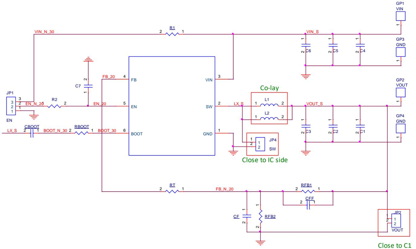
1. The capacitance values of the input and output capacitors will influence the input and output voltage ripple.
