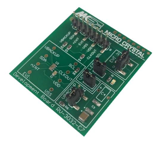
Temperature Compensated RTC Module
