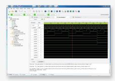
A signal-centric debugger that allows easy insertion of embedded logic analyzer for real time hardware debugging
