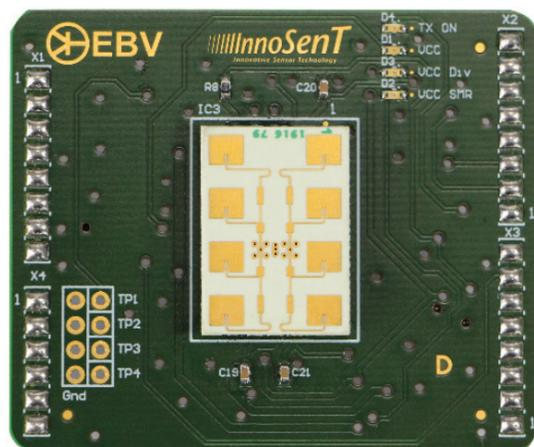
Figure 1: SMR Antenna module
