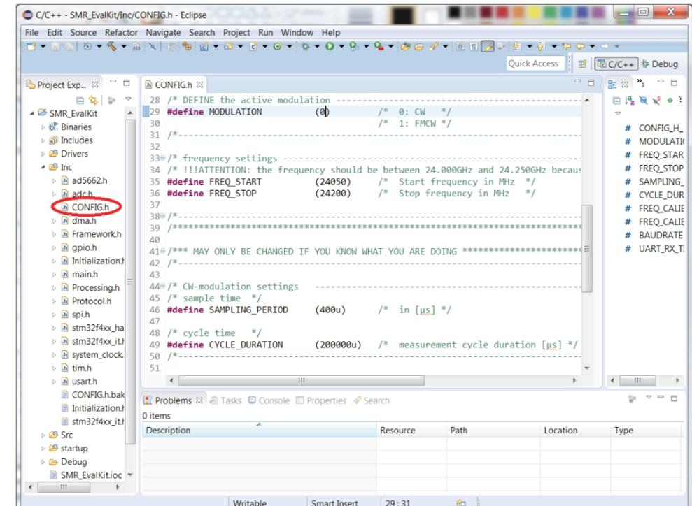
c) The radar setting can be changed by modifying the parameters in this "CONFIG.h" file. For example changing radar configuration to FMCW mode by setting "#define MODULATION (1) "
