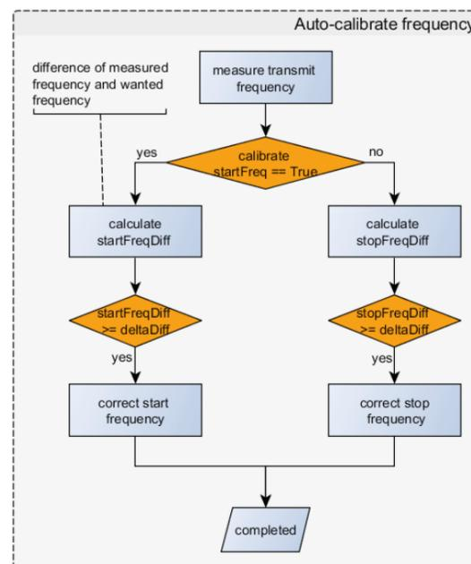
a) In the first step the transmit frequency of SMR module is measured. Afterwards the difference between the target transmit frequency and the measured transmit frequency is calculated. Based on this difference the transmit frequency is changed accordingly and tested again.
