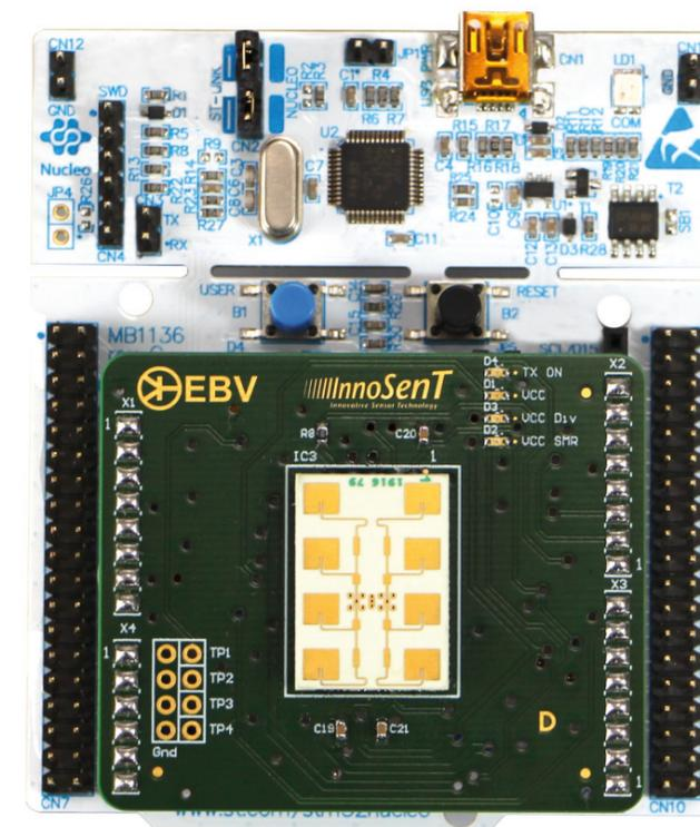
Figure 3: SMR-board and STM32 board connection
