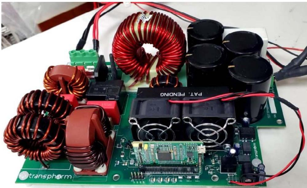
Figure 1. TDTP4000W066B\_0v1 4kW totem-pole PFC evaluation board
