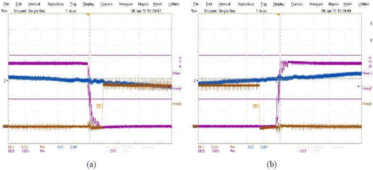
Fig 14 Zero-crossing transitional waveform (a) from negative to positive half-cycle (b) from positive to negative half-cycle. CH1: PW< Gate Signal for  $S_{D2}$ ; CH2:  $i_L$  waveform; CH3:  $V_D$  waveform.
