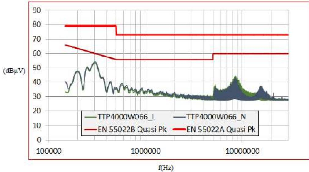
Fig 17. Conducted emissions @ 115V, 1150W
