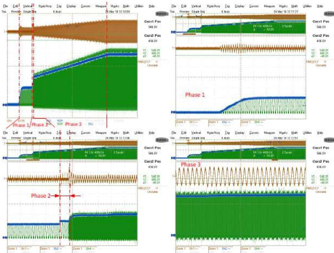
Fig 10. Start-up of the Bridge-less totem-pole PFC (CH1: lin, Ch2: Vo, CH3: Vds) with 1.2kW load
