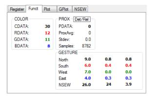
The Proximity indication shows the current reading (Raw Prox Count), a rolling average (ProxAvg), and the standard deviation of the rolling samples. The number of samples is specified on the Input Side. "Functional" tab.
