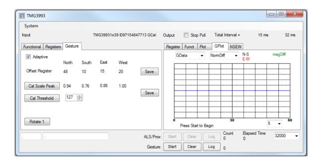
This window has inputs organized on the left, and outputs organized on the right. Values for register variables may be set using multiple techniques. The Functional tab is commonly used to quickly evaluate the device with nominal settings. The Input Register tab allows the register settings to be changed, and the Output Register tab allows registers to be viewed. Other tabs provide additional demonstration and test features for evaluation.
