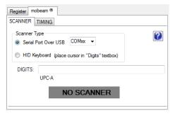
If an LS2208 (Serial emulation) scanner is used, then "Serial Port Over USB" must be selected and the appropriate COM port must also be selected in the "COMxx" dropdown box. Note that a USB driver must be installed for Windows OS to recognize the scanner.
