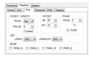
**Note:** Due to the automatic nature of the gesture algorithm, values entered in the registers and list boxes may not automatically update each other, so the values displayed may not match. The computed values on the right are always correct and show the values currently in use.
