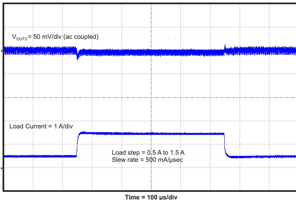
**Figure 10. TPS54495EVM Converter 2 Load Transient Response**
