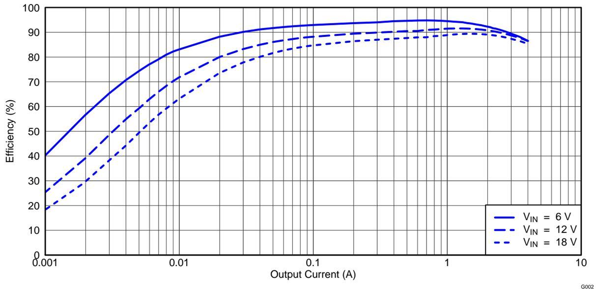
Figure 2. TPS54495EVM Converter 1 Light Load Efficiency
