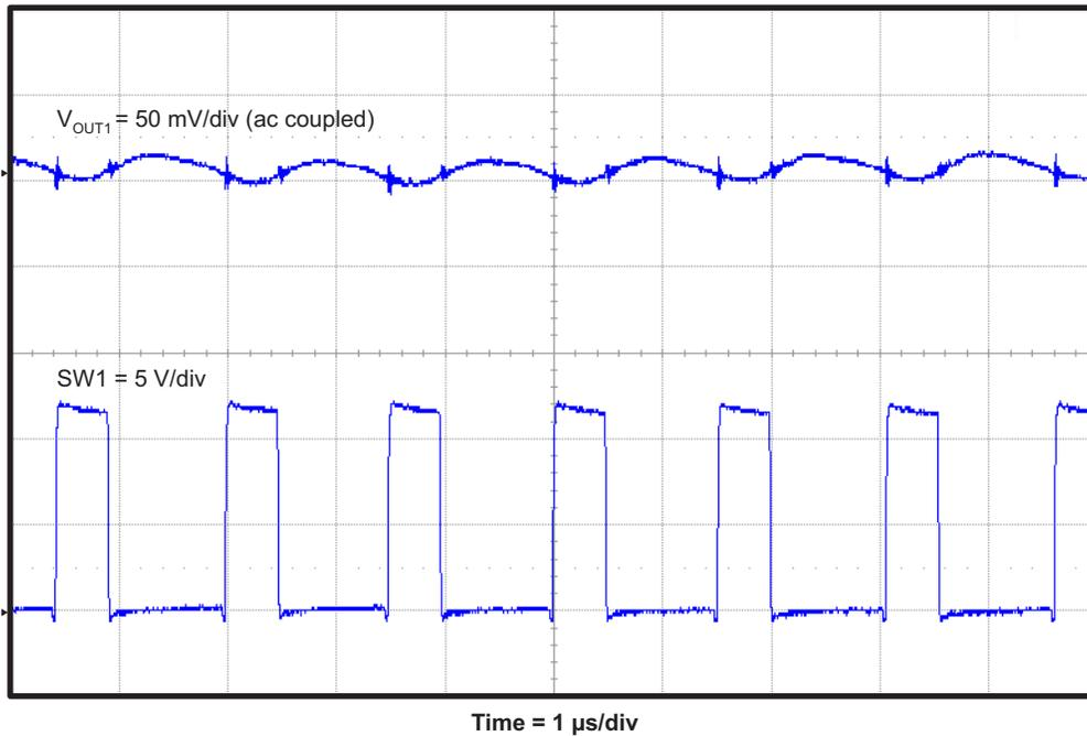
**Figure 11. TPS54495EVM Converter 1 Output Voltage Ripple**
