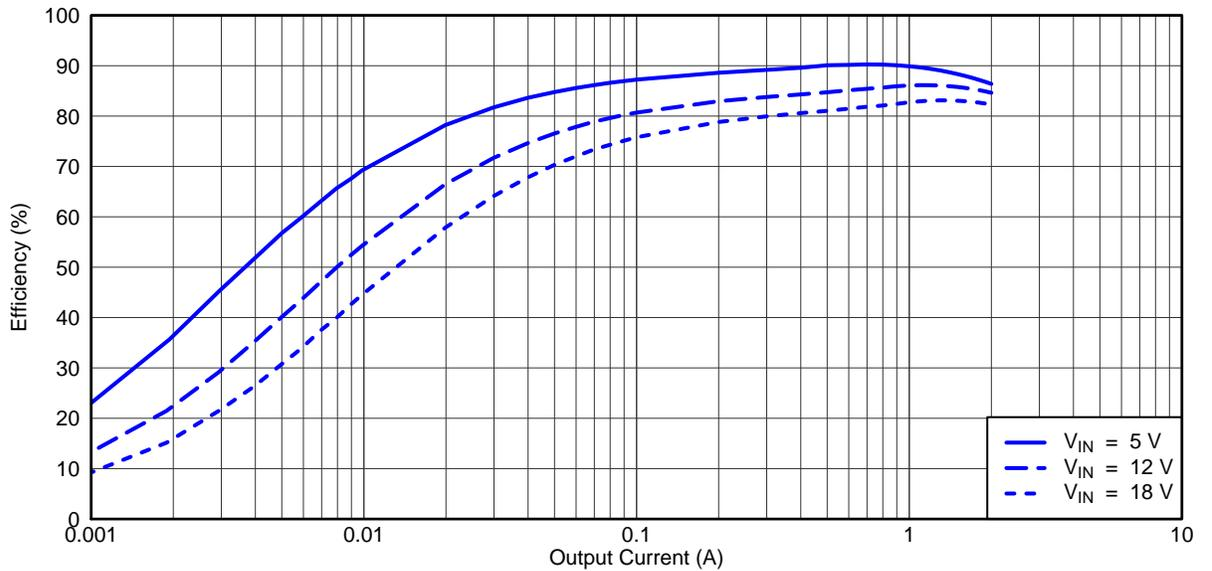
Figure 4. TPS54495EVM Converter 2 Light Load Efficiency
