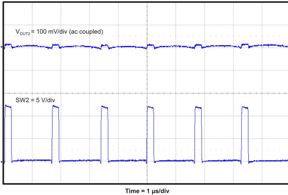
**Figure 13. TPS54495EVM Converter 2 Output Voltage Ripple**
