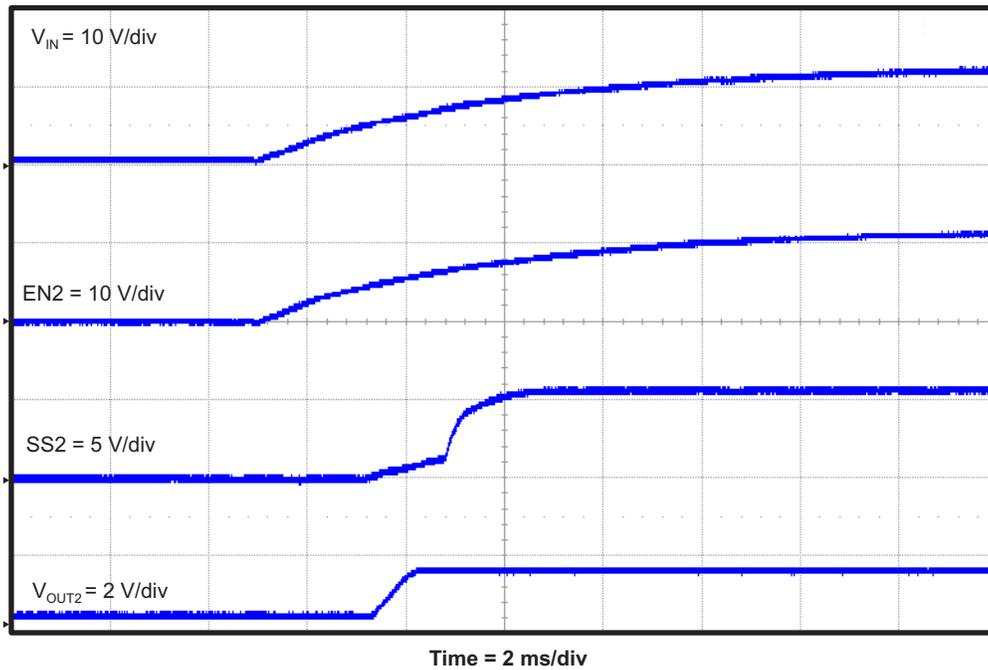
**Figure 18. TPS54495EVM Converter 2 Start-Up Relative to  $V_{IN}$**
