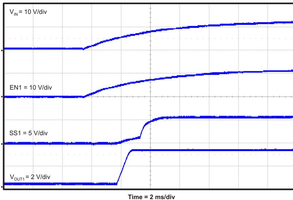
**Figure 16. TPS54495EVM Converter 1 Start-Up Relative to  $V_{IN}$**
