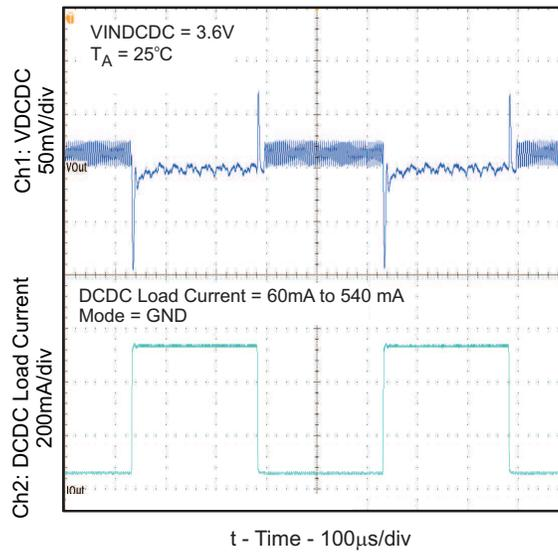
Figure 3. TPS650001/3/6 DCDC Converter Load Transient Response
