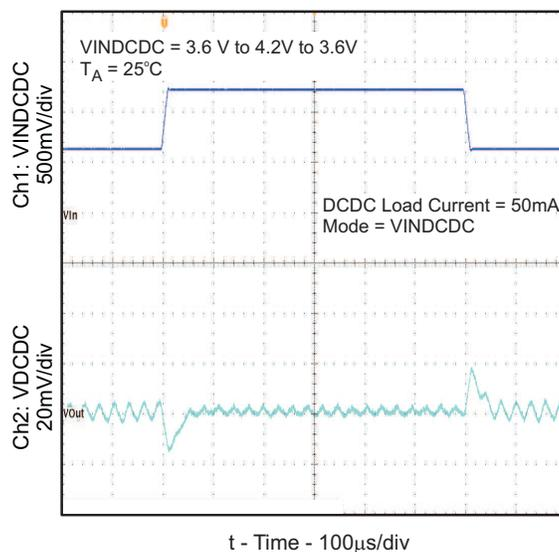
Figure 5. TPS650001/3/6 DCDC Converter Line Transient Response
