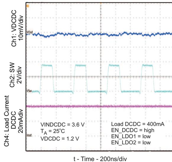
Figure 8. TPS650001/3/6 Output Voltage Ripple (MODE = high)
