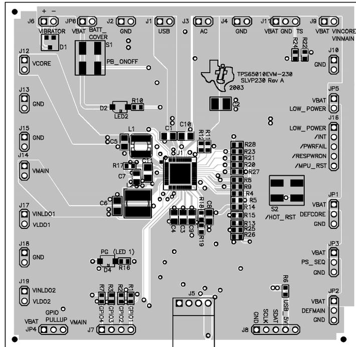
Figure 3-2. Top Layer Routing
