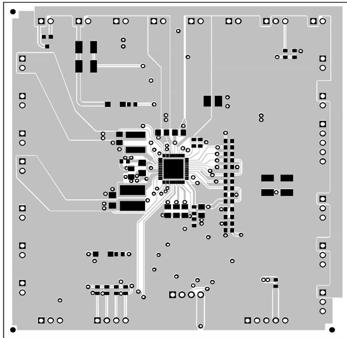
Figure 3-3. Layer 2 Routing
