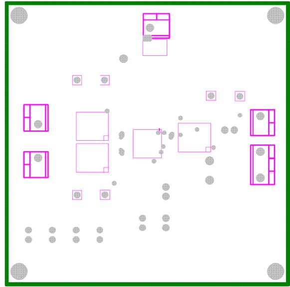
Figure 4. Middle Layer (2nd), Solid Cu Ground
