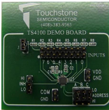
Figure 1. TS4100 Demo Board (Top View)
