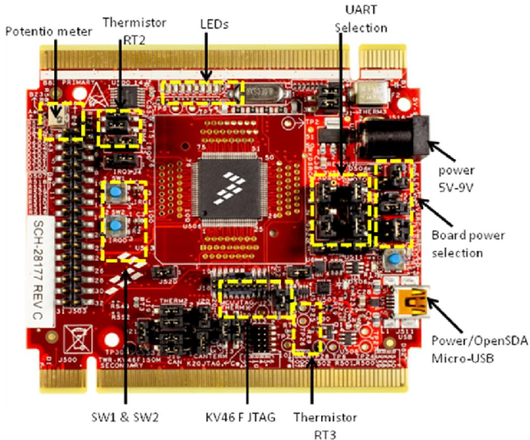
Figure 2. Front side of the TWR-KV46F150M module
