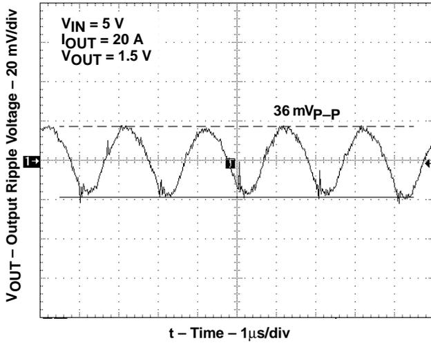
Figure 15. Output Ripple Voltage
