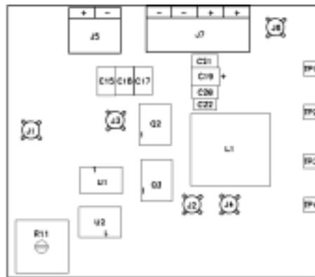
Figure 19. Top Side Component Assembly
