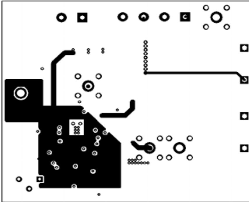
Figure 22. Internal Signal Ground and Trace Layer
