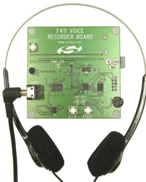
**Figure 1. Voice Recorder Reference Design Board**
