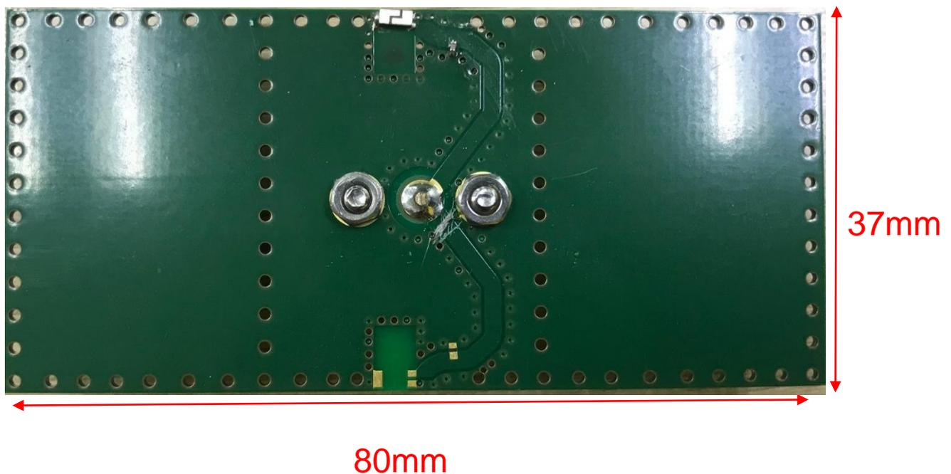
**Description:** 1.575 GHz GNSS Ceramic Chip Antenna
