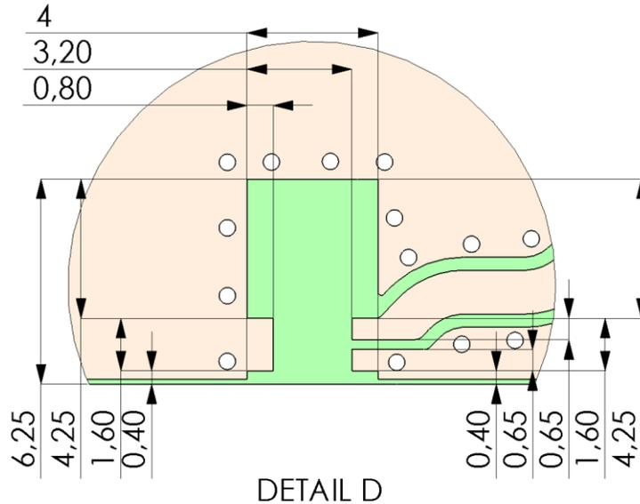
Antenna position on PWB layout
