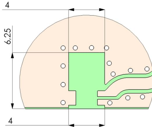
All metallization should be removed from all PWB layers on ground clearance area (4,00 x 6,25 mm).
