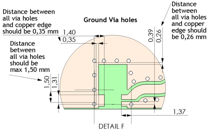
Solder resist opening and paste stencil recommendations for W3011A GPS Antenna
