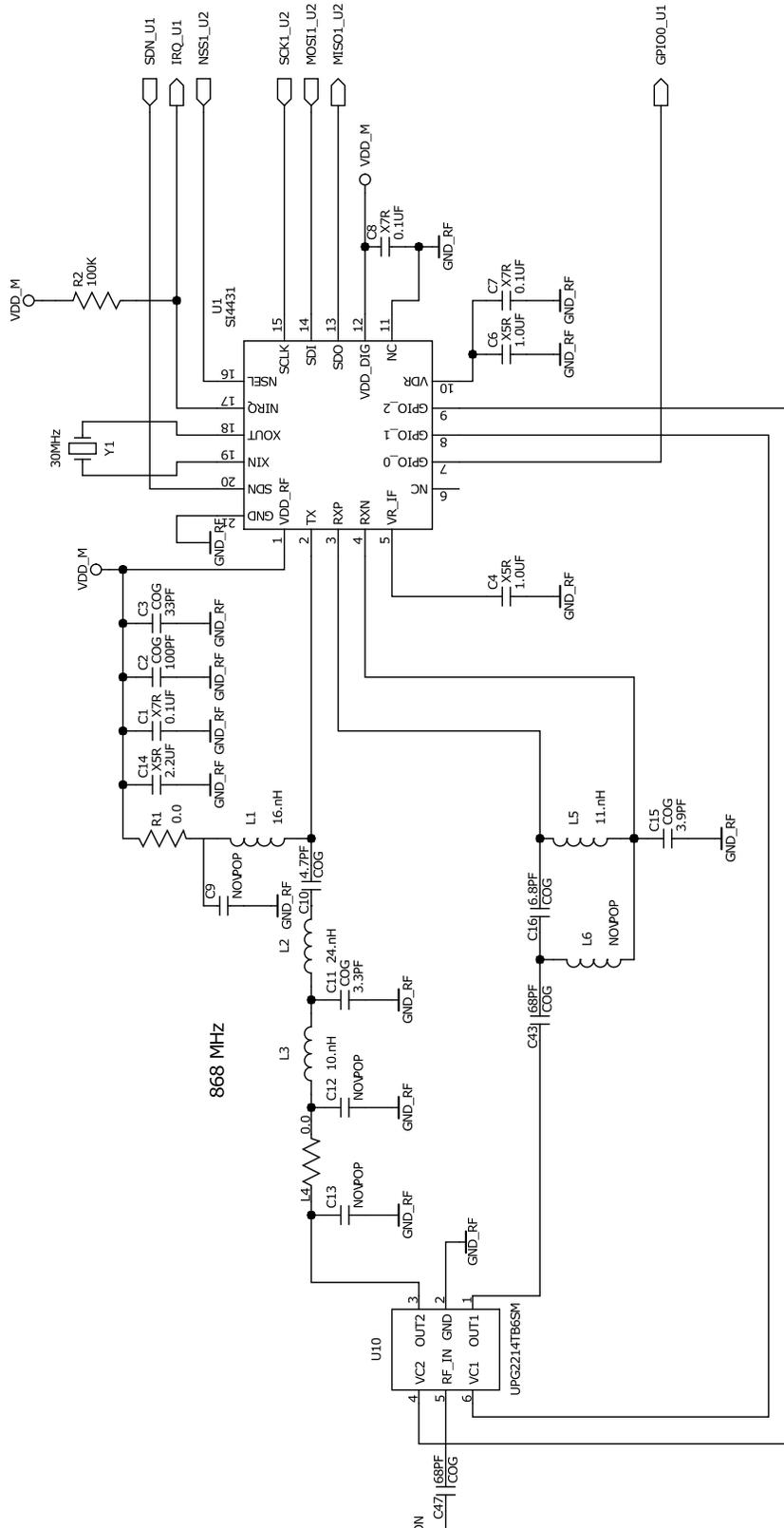
Figure 9. M-Bus Demo Board RF Section (1 of 4)
