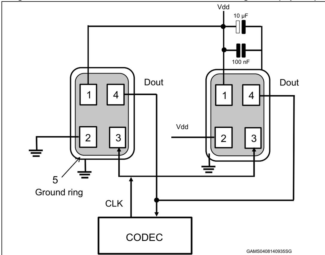
Power supply decoupling capacitors (100 nF ceramic, 10  $\mu$ F ceramic) should be placed as near as possible to pin 1 of the device (common design practice).
