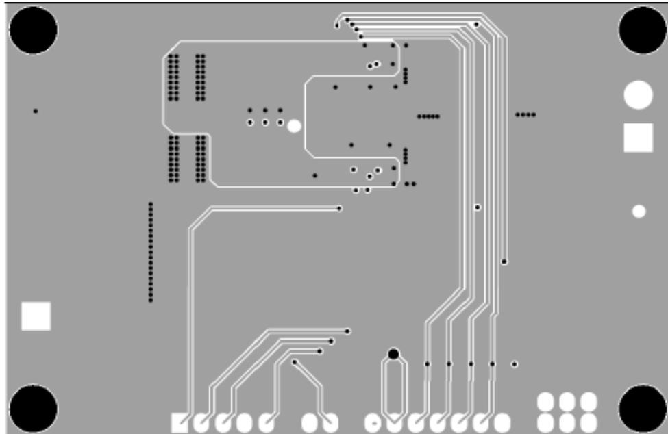
Figure 7. 6038-443.16 - FDA803D (903D) – Bottom layer and silkscreen
