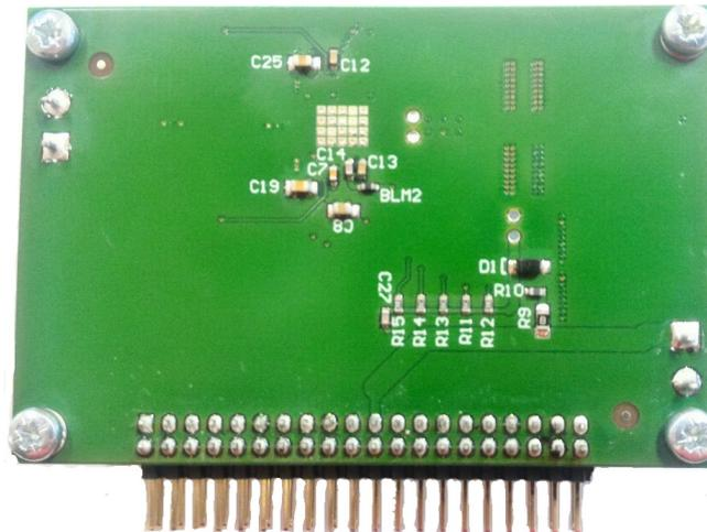
Note: The output LC filter in this module can be assembled with different values and kind of coils and capacitors. By default it is assembled for a 14.4V application with ferrite coils that are a good compromise considering performances, price and availability that allow to drive 4 ohm.
