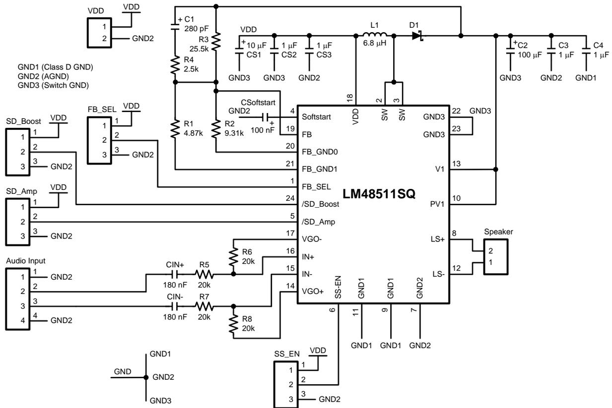
Figure 2. Typical LM48511 Audio Amplifier Application Circuit
