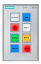
SIMATIC HMI KP8 PN Key Panel, 8 short-stroke switches with multi-colored LEDs, PROFINET interfaces 8 configurable DI/DO pins, 24 V DC can be looped through parameterizable as of STEP 7 V5.5
