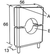
Hole center spacing: A=ø 45
