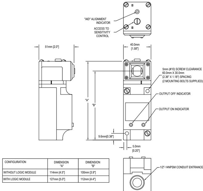
Figure 4. Dimensions for the fiber models
