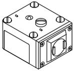
Fixed-field sensor heads have an emitter element and two differently-aimed receiver elements. This creates a high-gain sensing field able to detect objects of low reflectivity, and a sharp far-limit sensing cutoff of 50mm (2 inches) or 100mm (4 inches) which ignores backgrounds beyond cutoff.
