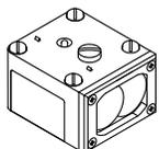
MAXI-BEAM emitters have a visible red "tracer beam". This beam is non-active, and is used as a means of visual alignment during installation. A retroreflector temporarily attached to the receiver lens provides an effective target for the tracer beam during alignment. The narrow beam of the RSBESR/RSBRSR pair is ideal for sensing small parts (effective beam diameter is 3.6 mm (0.14 in)).
