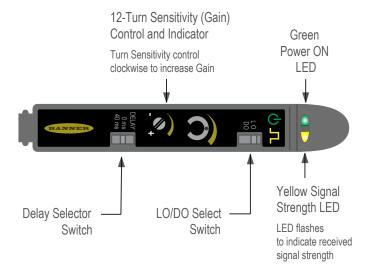
In dark operate (DO) mode, the output is ON when the target returns less light to the sensor than the configured target and OFF when the sensor detects more light than the configured/taught target. In light operate (LO) mode, the output is ON when the target returns the same or more light to the sensor and OFF when the sensor detects less light than the configured/taught target.
